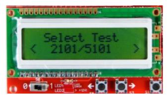
If the LCD screen is blank then the contrast needs adjusting. Using a small screwdriver, slowly rotate the potentiometer counter clockwise until text appears on the LCD screen.
