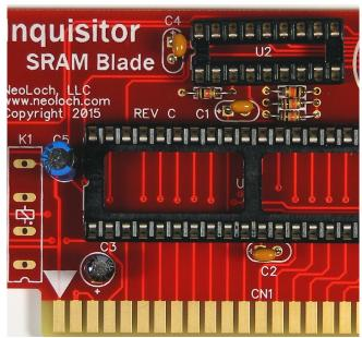
**Step 7:** To Solder the reed relay into K1 you'll need to take care as the relay has a built in suppression diode, so the relay is polarized.
