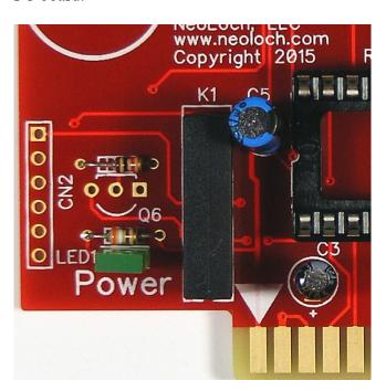
The relays will make a low clicking sound when being turned off. If the tester isn't working as it should after assembly is complete, listening for this click can help troubleshoot the relays as a possible cause.
