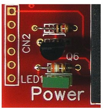
**Step 10:** Solder in the remaining transistors into Q1 through Q5. And Q7 for SRAM II PCB (not shown).
