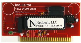
This completes the assembly of the 4116 blade. Now you can insert the blade into the Inquisitor core module and test the blade to make sure everything is working as intended.
