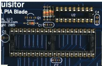
**Step 5:** Solder the 0.1uF capacitors into C1, C2 and C4.
