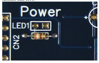
**Step 2:** Solder a  $1K\Omega$  (Brown, Black, Red) resistor into R4.
