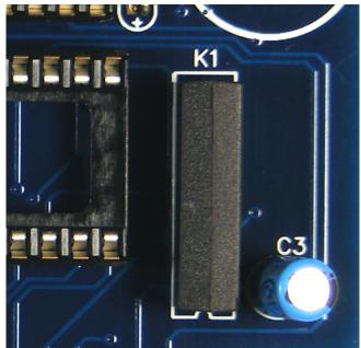
The relays will make a low clicking sound when being turned off. If the tester isn't working as it should after assembly is complete, listening for this click can help troubleshoot the relays as a possible cause.
