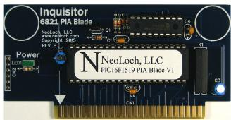
This completes the assembly of the PIA blade. Now you can insert the blade into the Inquisitor core module and test the blade to make sure everything is working as intended.
