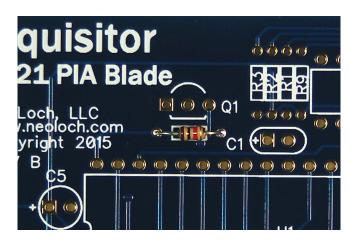
**Step 3:** Solder the  $10K\Omega$  (Brown, Black, Orange) resistors into R1, R2, R3 and R9.
