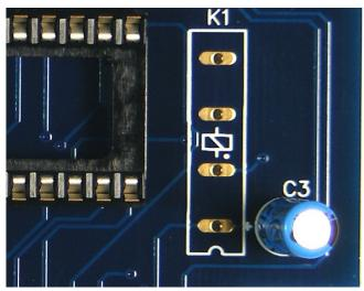
**Step 8:** To Solder the reed relay into K1 you'll need to take care as the relay has a built in suppression diode, so the relay is polarized.
