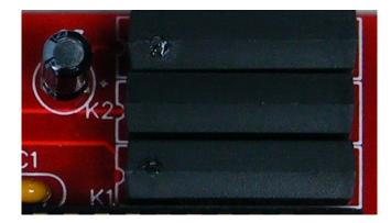
To Solder the reed relay into K1, K2 and K3, you'll need to take care as the relay has a built in suppression diode, so the relay is polarized.
